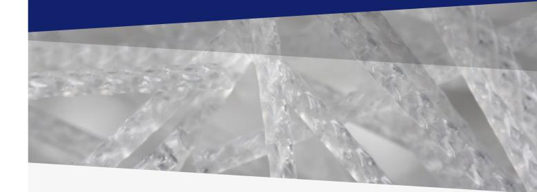
Durus \$400 is a macro synthetic fibre that is extruded, embossed and then specifically cut into the lengths required for each concrete application. Durus \$400 is used in readymix, precast & sprayed concrete applications. The embossment improves the bond between the fibre and the concrete resulting in improvements to the residual flexural strength of the concrete.
